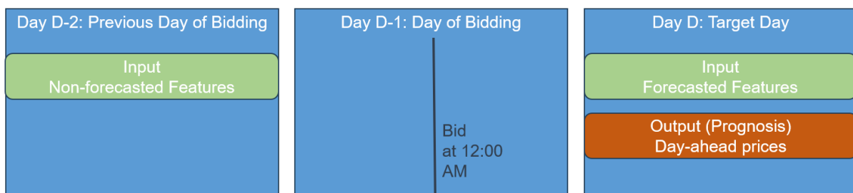
Figure 3: Forecasting setup for the target variable "day-ahead prices"
