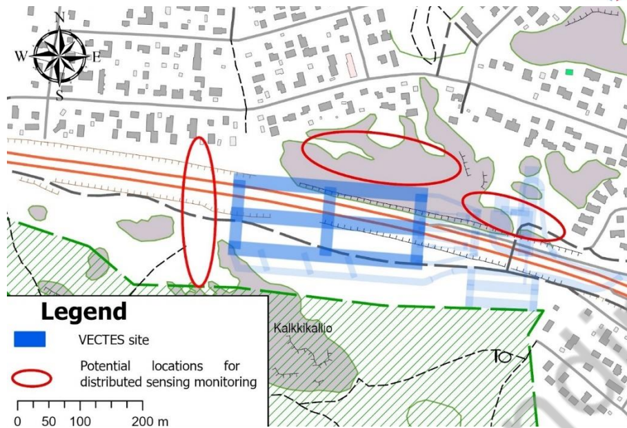
Figure 19. Potential locations for distributed sensing measurements around the VECTES caverns. The fibre optic cables can be installed in the caverns after the excavations have been completed.
